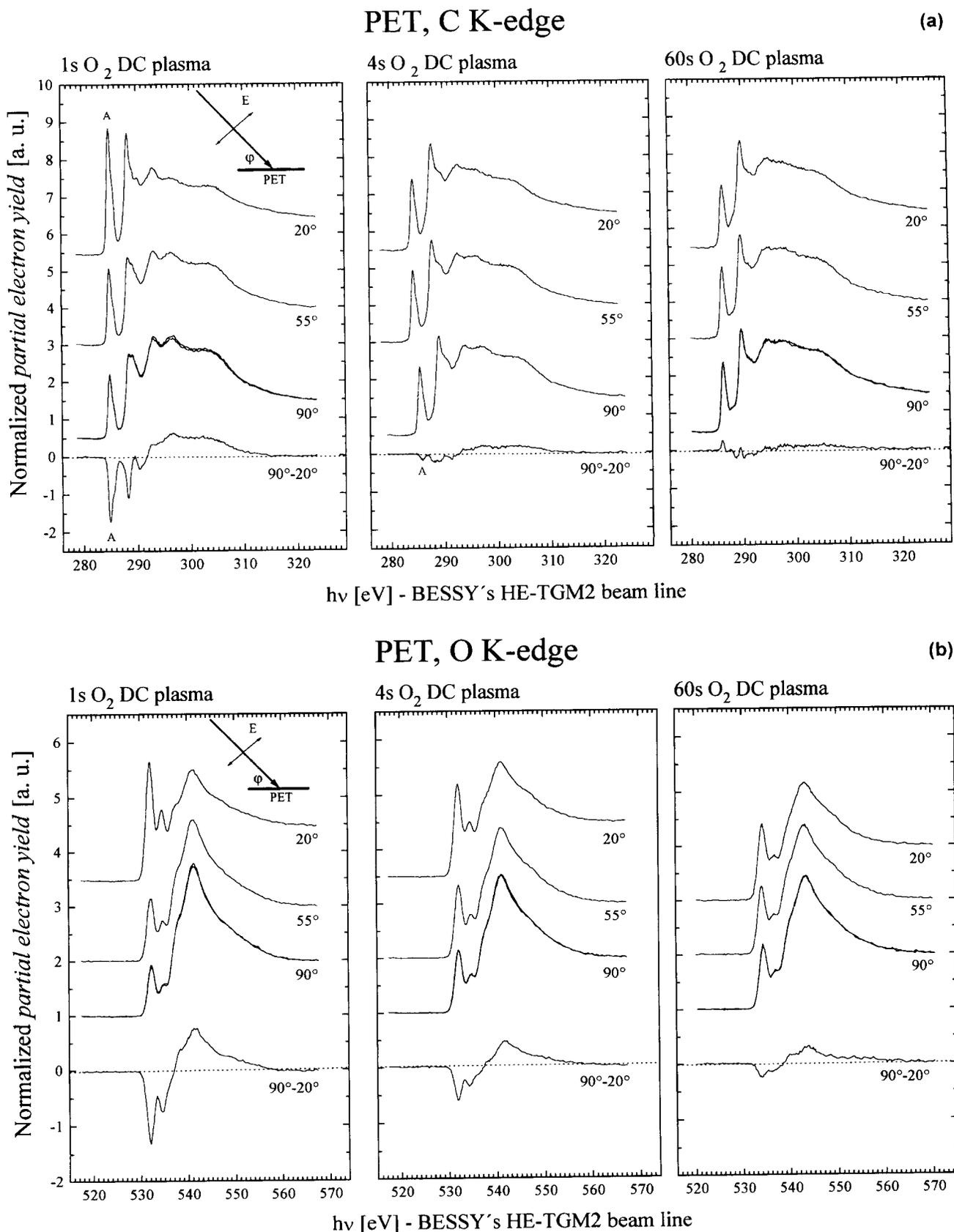
**Figure 2** Angle resolved normalized PEY (a) C and (b) O K-edge X-ray absorption spectra of biaxially stretched PET foils after low pressure-oxygen d.c. plasma treatments
