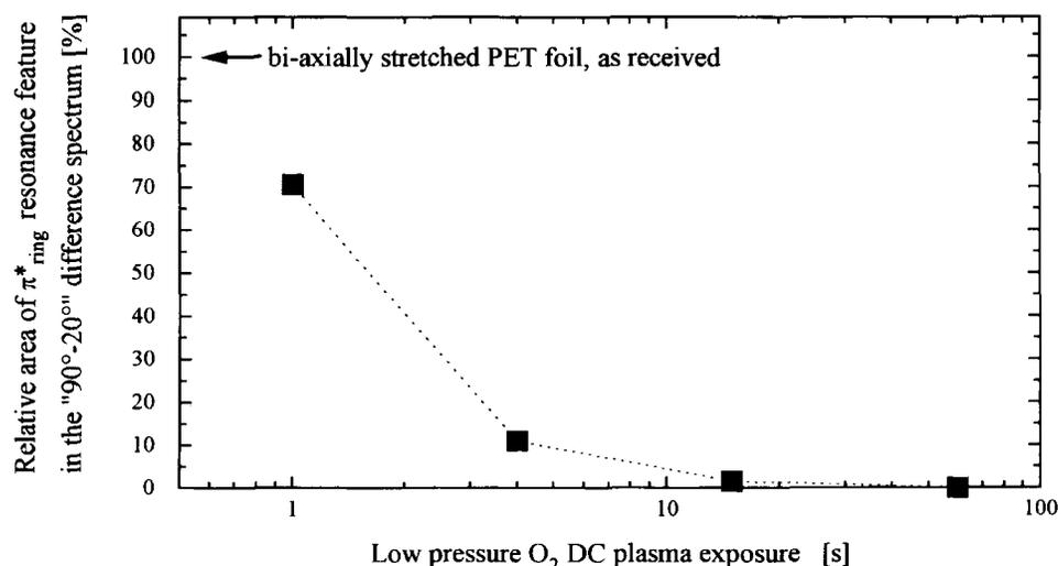
**Figure 3** The decrease of the area of the C 1s  $\rightarrow \pi_{\text{ring}}^*$  resonance related feature (A) in the C K-edge difference spectra of low pressure oxygen plasma treated biaxially stretched PET foils relative to the 'as received' state
